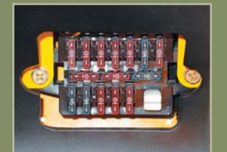
A concentrated fuse box for easy inspection
